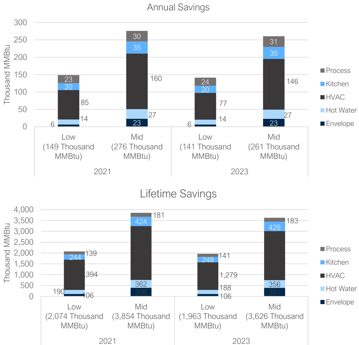
Figure 30. Non-Residential Annual and Lifetime Natural Gas Savings by End Use, Low and Mid Scenarios
